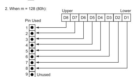
Note • When registering 7 x 9 fonts, dots adjacent in the horizontal direction do not print.
