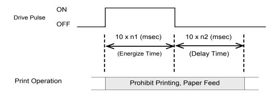
After printing, this is executed by BEL (External device 1 drive instruction) or FS (External device 1 drive instruction (real time)).
