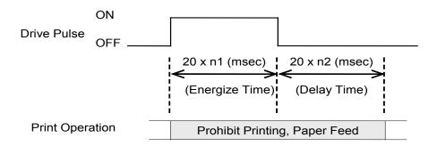
The drive of the external buzzer set by this command is performed by <ESC> <GS> <EM> <DC2> m n1 n2. The set value is not initialized by <ESC> "@", or <CAN>.
