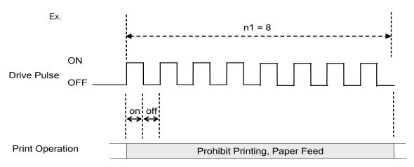
(Note) When off time = 0, it is possible to ring the buzzer continuously for only the amount of n1. For example, if on = 5 seconds, and off = 0, n1 = 20 times, the buzzer will ring for 100 seconds.
